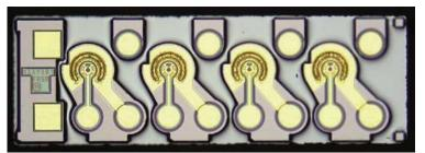
The V850-2106-001 and the V850-TBD-001 are high-performance 850 nm VCSEL (Vertical Cavity Surface-Emitting Laser) array die optimized for highspeed data communications. The array die are ideal for use in manufacturing transceivers for parallel optical interconnects. The arrays are available in either 4 or 12 channel configurations.
